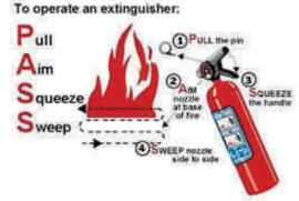
Fig. 3.3.10 Method of operating fire extinguisher
